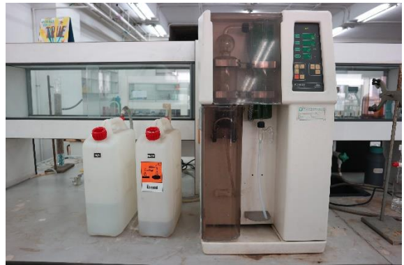
Distillation Unit (Ammonia),
