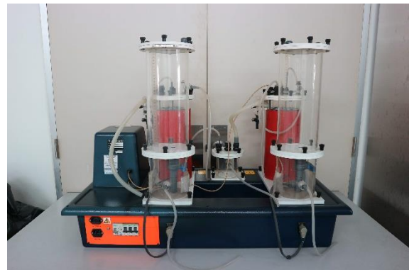
Aerobic treatment unit
