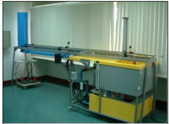
Water Hammer Test Set
