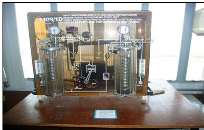
Demonstrative Refrigeration Study Units
